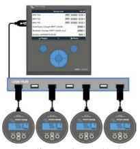
A maximum of four BMVs can be connected directly to the Color Control. Even more BMVs can be connected to a USB Hub for
